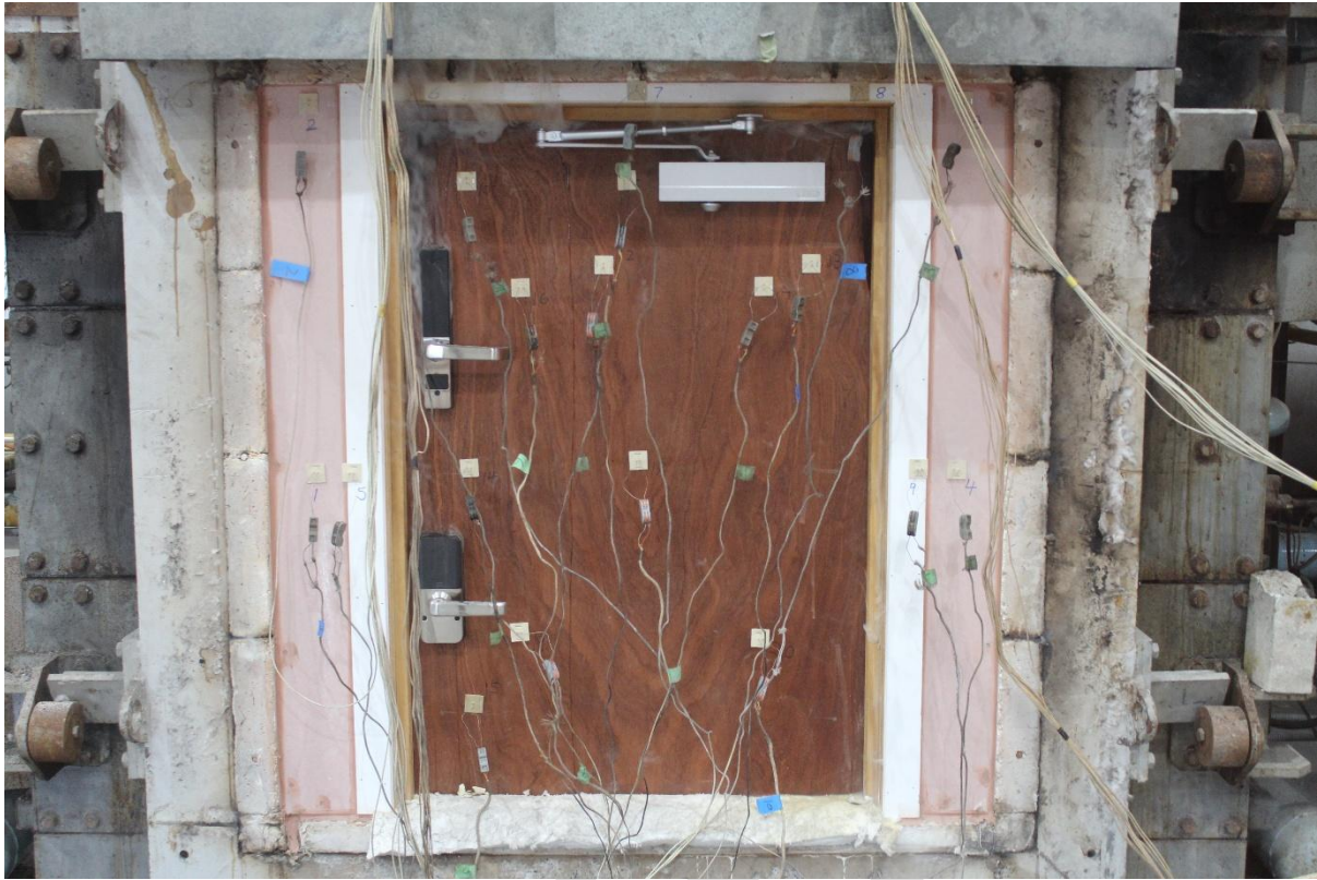
Figure 21 – Unexposed face at 15 minutes
