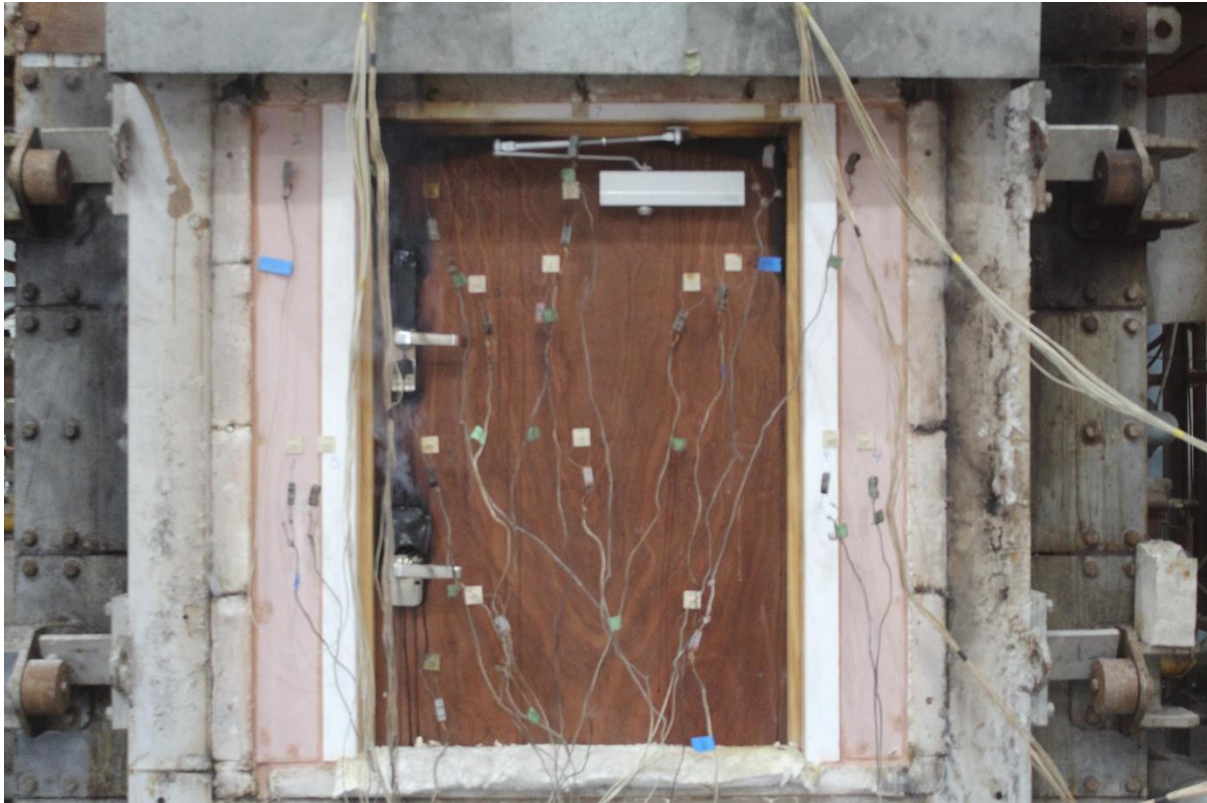
Figure 25 – Unexposed face at 60 minutes
