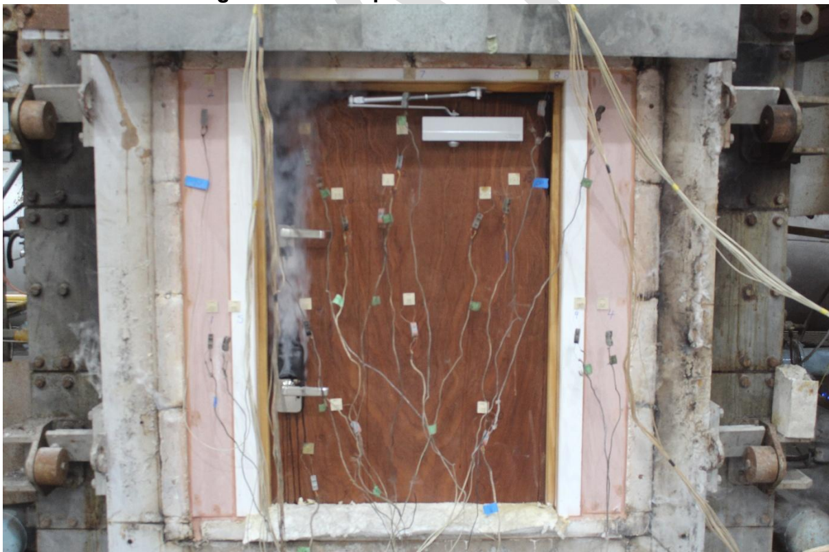
Figure 24 – Unexposed face at 45 minutes
