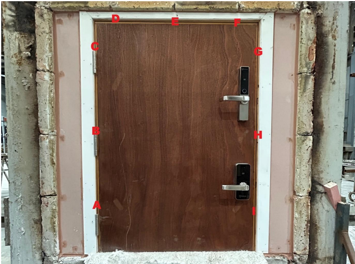
Figure 1 – Gap Measurement Location
