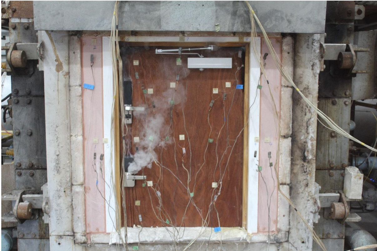
Figure 23 – Unexposed face at 30 minutes
