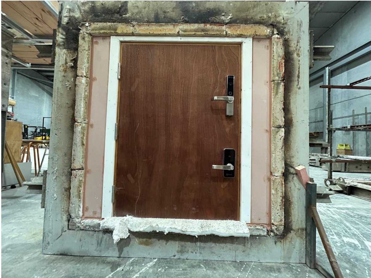
Figure 13 – Exposed face prior to test commencement
